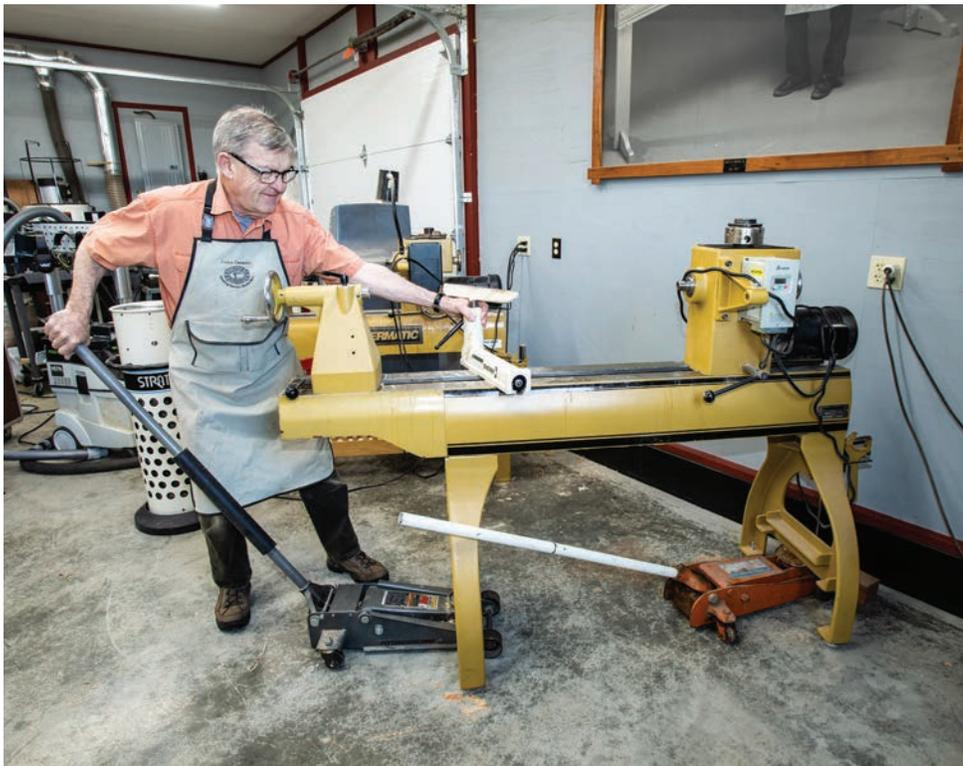
**H**ow the heck do you move a full-size lathe into a workshop in the first place, especially if it's in a basement? Well, if you think getting a big lathe down *into* a basement is daunting, moving a used one *out of it* is even more challenging! But, take heart: it's very do-able. My "More on the Web" video to support my August 2020 article ([woodworkersjournal.com](http://woodworkersjournal.com)) should help, and I offer some tips for moving heavy woodworking machinery in general.
