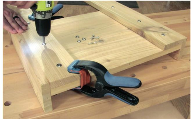
5. Cut the bottom supports to length and attach them to the bottom of the panels with 2" screws.
