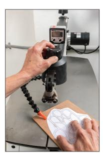
5. Problem: Excess burning when cutting thick or dense wood. *Possible causes*: wrong size or type of blade for thickness or type of wood.
