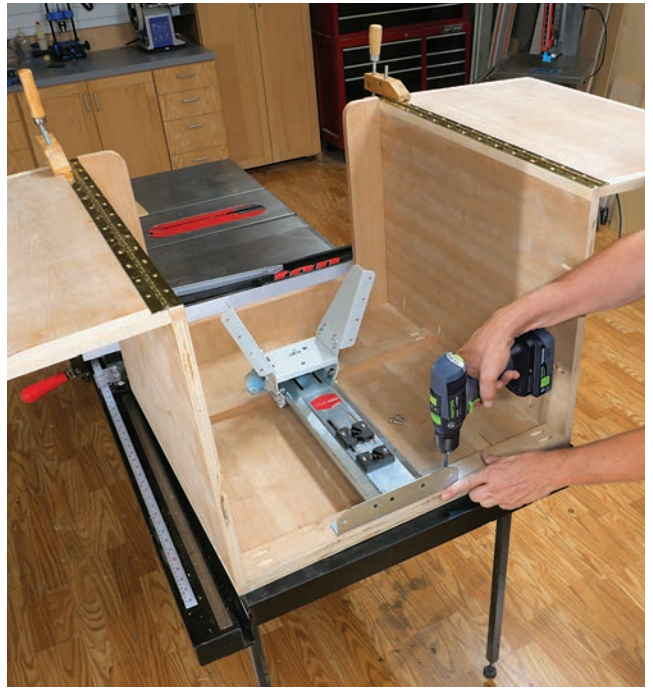
Install a pair of plywood lift supports inside the cabinet (left). Then attach the sewing machine lift hardware to the supports (right). The lift is adjustable to accommodate almost all sewing machines. Here the cabinet's top work surface is removed for clarity.
