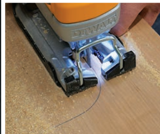
The bottom (Piece 2) has a large foot recess to cut away. Lay out this shape using the Drawing on page 37. Common shop supply containers like cans or glue bottles can provide the curves you need to draw the shape easily. Cut the recess with a jigsaw (inset).
