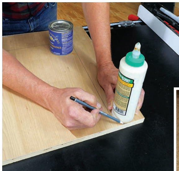
The bottom (Piece 2) has a large foot recess to cut away. Lay out this shape using the Drawing on page 37. Common shop supply containers like cans or glue bottles can provide the curves you need to draw the shape easily. Cut the recess with a jigsaw (inset).
