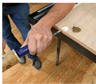
The author created a jig (left) to mortise for the sewing machine hinges. These hinges must be flush to the top of the work surface. After the hinge mortises are routed out, use a sharp chisel to create a deeper recess for the hinge knuckles (inset).
