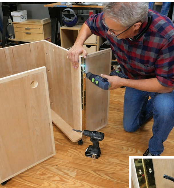
Mounting and aligning doors on piano hinges is a fussy but achievable task. A self-centering drill bit (inset) makes installing the hinges' many screws easier.
