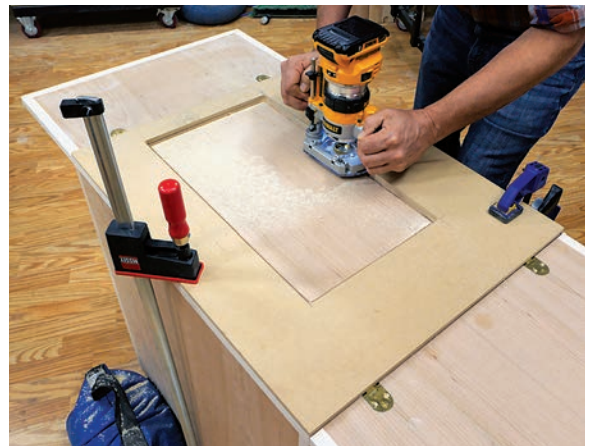
Rout out the sewing machine platform from the top/work surface using a 1/4" straight bit. An MDF cutting guide provides a reference edge for the router's 5/16" guide collar to follow.
