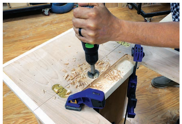
The cabinet's brass grommet must sit flush to the work surface, which requires a two-step machining process and two Forstner bit sizes.
