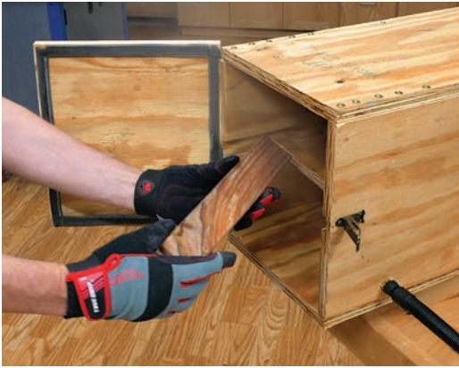
Take care when removing stock from the steam chamber — it is very hot. Note the slat inside the chamber to hold the stock in the middle of the steam.
