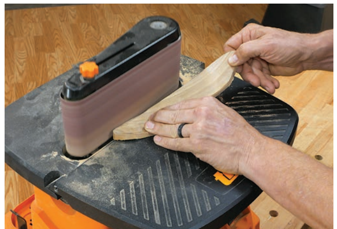
Use a stationary belt sander or disc sander to smooth the curves and do any final shaping. Sand the coat hooks smooth before applying a finish.
