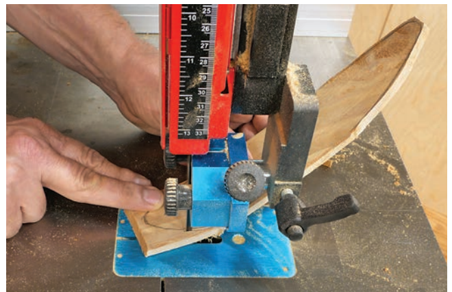
Cutting out the coat hook shape on the band saw requires special attention. Rotate the stock so that the section being cut is flat on the table, and cut carefully. A 1/4" blade is a good choice for cutting these tight curves.
