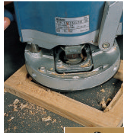
Figure 2: The size of the rabbeting bit and bearing is critical. The goal here is to fit a square cornered piece of glass into an opening with rounded corners.
