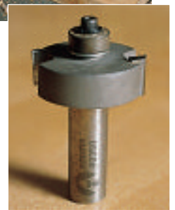
Figure 2: The size of the rabbeting bit and bearing is critical. The goal here is to fit a square cornered piece of glass into an opening with rounded corners.
