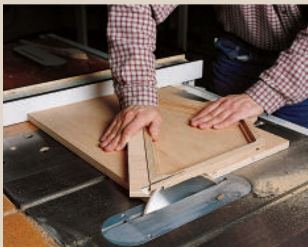
The first jig miters the left side of the frames.
