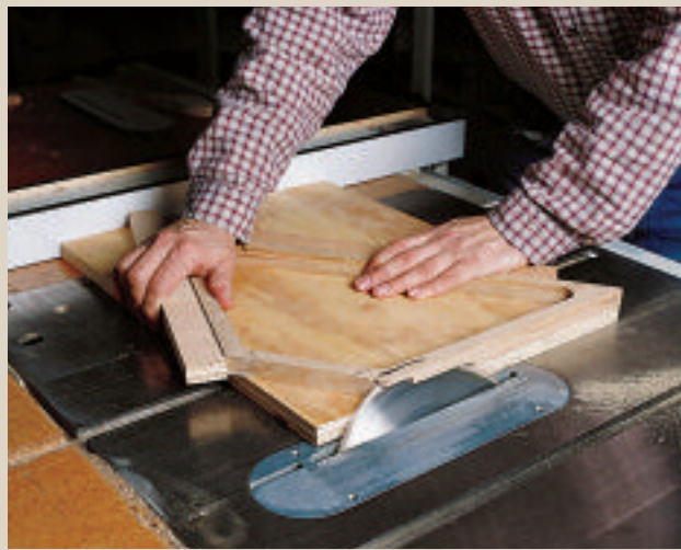
The second jig miters the right sides.
