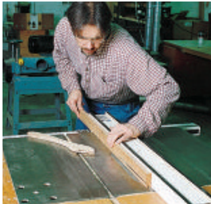
Figure 1: Make sure your rip fence is positioned opposite the direction the blade tilts when making the first two chamfers on the base molding.
