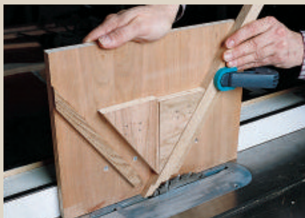
Figure 3: With the same dado blade in your table saw, use our jig to help chop the mortises and slice the tenons on the ends of the frame's stiles and rails.
