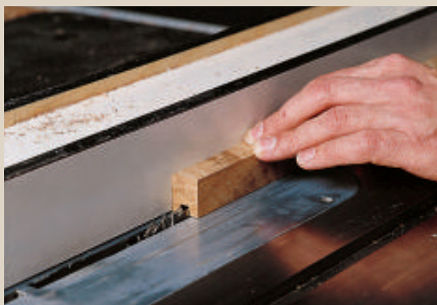
Figure 2: Before cutting the rails and stiles to length, use a dado blade to plow a groove. This will make it easier to create the rabbets for the glass after you assemble the frames.
