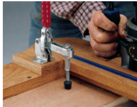
Figure 3: The hold-down clamp is mounted on a spacer block and modified with a 1"-long hex head bolt and a connector nut.
