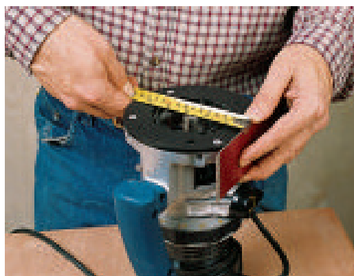
Figure 1: Determining the space required for your router is critical to the success of this jig. Measure your router and the two pieces of laminate to get the exact dimension.
