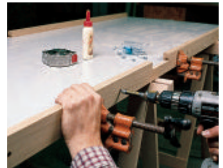
Figure 2: Attach the rails to the melamine deck with screws and glue. Cover the exposed screw holes with walnut plugs.
