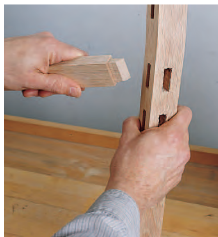
Figure 1: Mortise and tenon joinery is the key to this chair's durability. Different mortise locations create right and left chair parts. Some of the tenons are mitered to meet inside the uprights.
