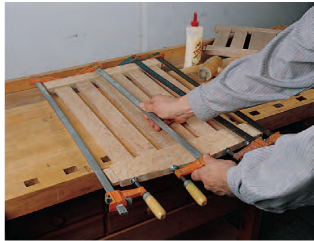
Figure 2: Glue up the subassemblies of the back and chair sides. Make sure they are flat and square. After the glue has cured, move on to the final assembly.
