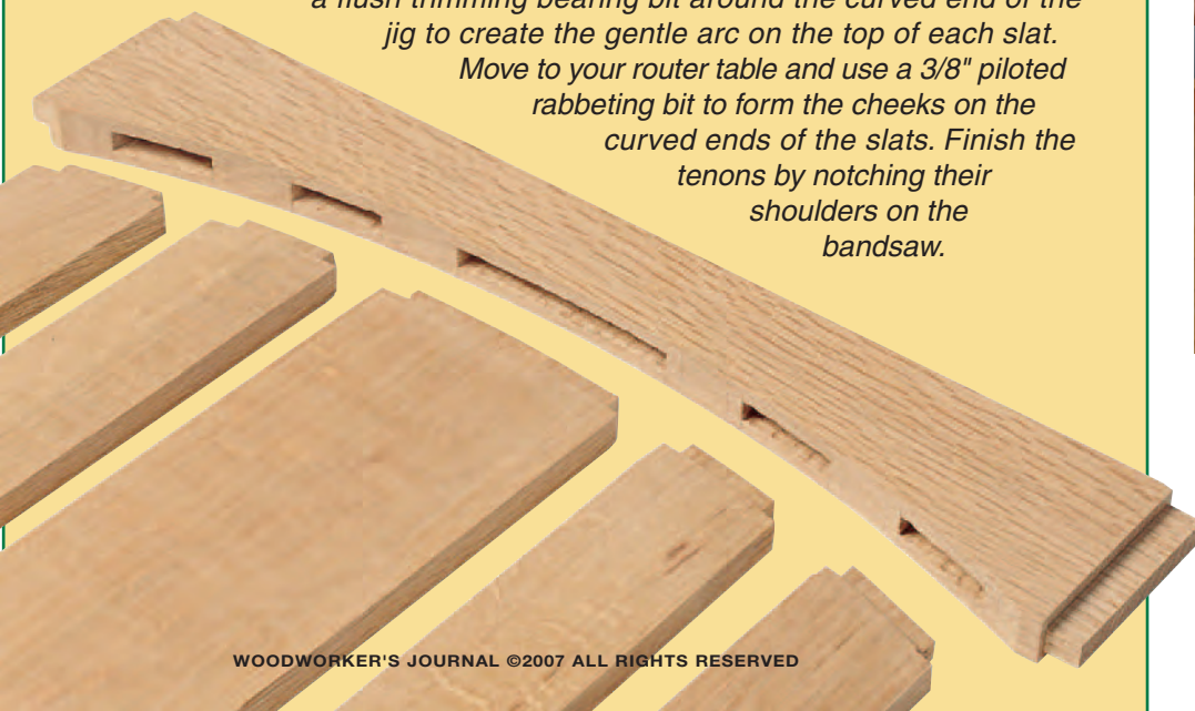
Figure 1: Mortise and tenon joinery is the key to this chair's durability. Different mortise locations create right and left chair parts. Some of the tenons are mitered to meet inside the uprights.
