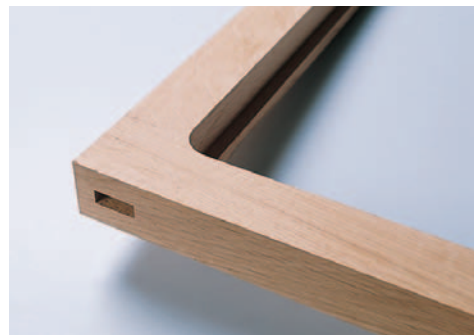
Figure 2: Assemble the desktop frame and cut a rabbet in its bottom edge with a bearing-guided bit. Square the corners with a sharp chisel.
