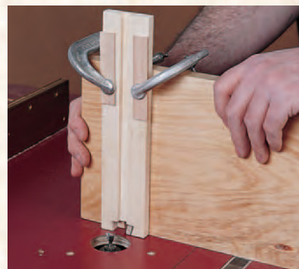
Figure 3: Use a high auxiliary fence on the miter gauge to cut the dovetail pins on the drawer sides. A dovetail saw can be used to cut the tails (right) on the drawer fronts.
