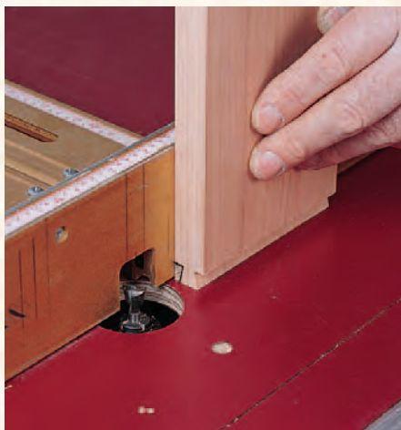
Figure 2: Use scrap cutoffs from the apron stock (since they're the exact thickness of your workpieces) to set the fence for the dovetail cuts on the aprons.
