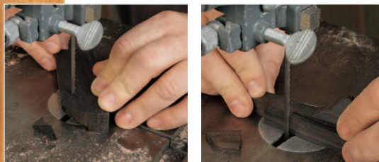
For the solid-ebony pulls, first create a molding as shown in the Drawings . Complete the pulls' organic shape on the band saw and disk sander.
