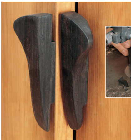
For the solid-ebony pulls, first create a molding as shown in the Drawings . Complete the pulls' organic shape on the band saw and disk sander.
