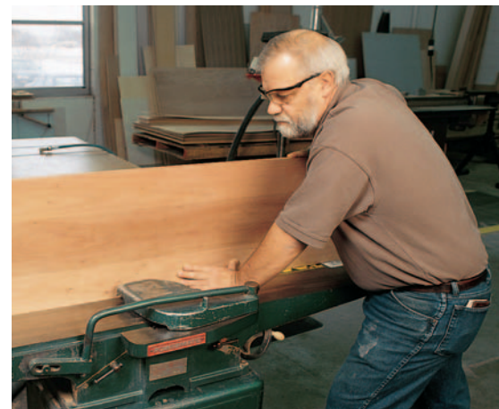
Joining a dead-straight edge on the 1" thick glued-up side blanks is the first step in accurately machining the carcass.
