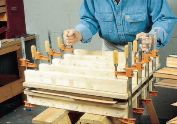
Laminate the door layers in a shop-made veneer press. The waxed platens resist glue and the clamping cauls and battens transfer pressure to the glue-up. You can gently crown the battens or just glue a small section of veneer at the center of each batten.
