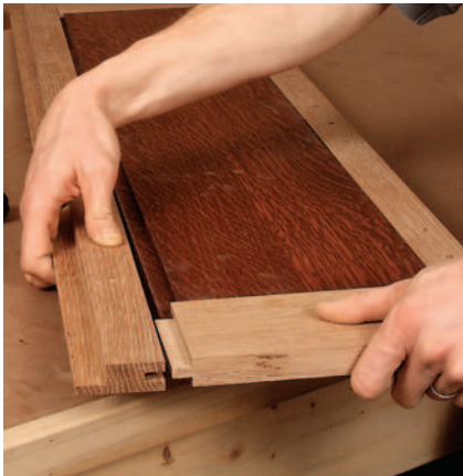
Tongue-and-groove joints connect the upper cabinet end frame parts. Finish the floating panels before assembling these frames.
