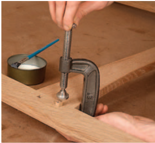
Make the face frame pegs from longer strips, chamfering each on a sander before cutting it to length. A simple angle jig helps maintain even chamfers. Press the pegs into their square face frame holes with a C-clamp to avoid marring them.
