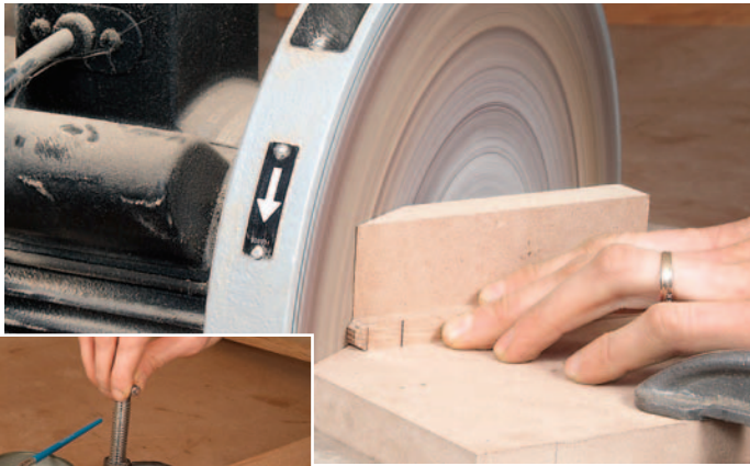
Make the face frame pegs from longer strips, chamfering each on a sander before cutting it to length. A simple angle jig helps maintain even chamfers. Press the pegs into their square face frame holes with a C-clamp to avoid marring them.
