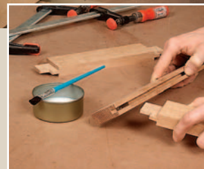
Nibble the haunched portion on the tenons so they'll fit into their mortises on the door stiles. A 1/2"-thick spacer on the rip fence establishes the haunch length.
