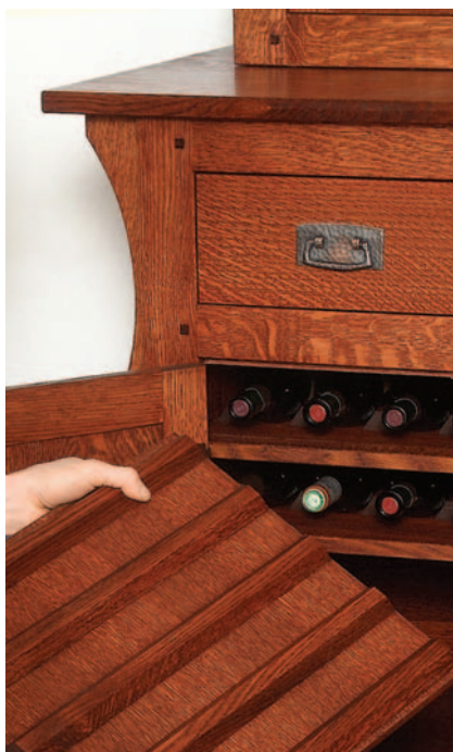
Removable shelves in the base cabinet are outfitted with divider strips to keep the bottles stationary and evenly spaced. The shelves could be flipped over onto their flat faces for storing other items as well.
