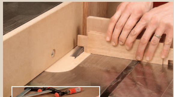
Nibble the haunched portion on the tenons so they'll fit into their mortises on the door stiles. A 1/2"-thick spacer on the rip fence establishes the haunch length.
