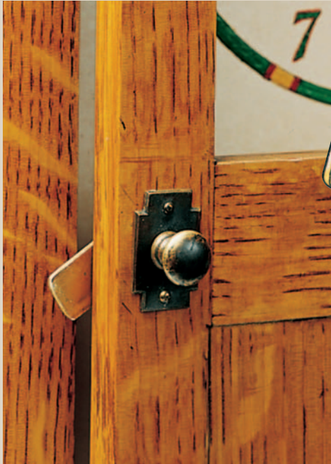
The author made his own hardware for this clock from some common metal supplies. Other pre-made door latches would also work here.
