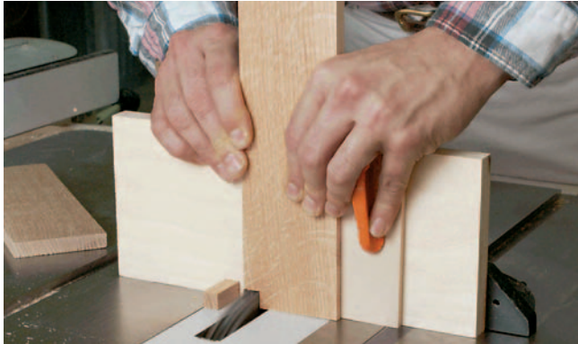
To help form the box joints, attach a simple fence with a registration key to your miter gauge. Always test your cuts on scrap. This setup will generally require some fine-tuning for proper alignment.
