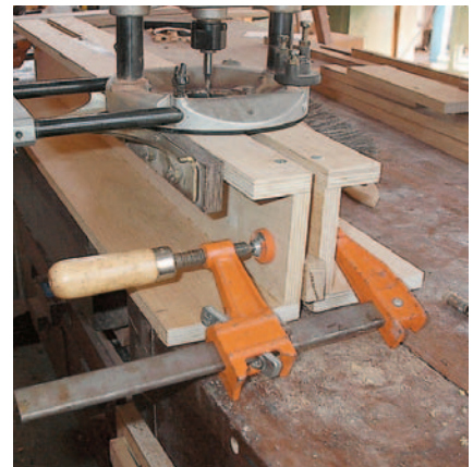
Two "L"-shaped fixtures can hold the door and face frame components securely for routing the "skinny" face frame mortises.
