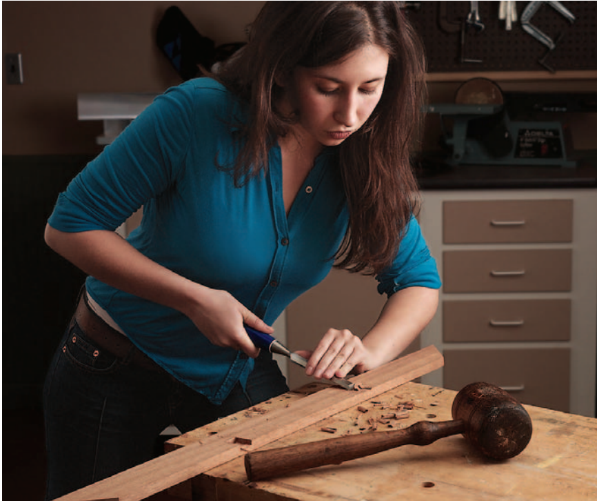
Since there are only four mortises to chop, lay them out and cut them by hand. The support rail's top edge must align perfectly with the rabbet on the tray stiles and rails.
