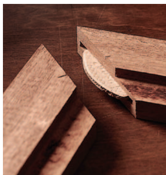
A biscuit or plate joiner is a great way to strengthen and align miter joints. The biscuits fit just under the tray's rabbet.
