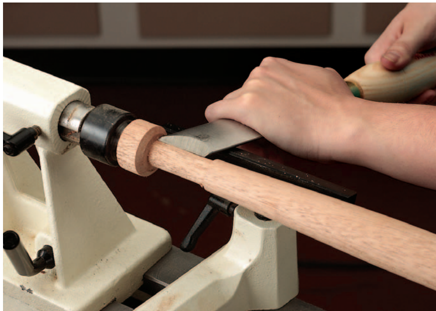
The turned tenons on both ends of the stretcher need to be long enough to engage both legs, on each side of the table, as you assemble the project. Use a skew chisel at the lathe to perfect their length and diameter.
