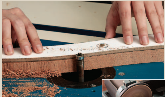
Use double-sided tape and one screw at the tenon mortise location to attach the template to a roughed-out leg. A flush-trimming bit shapes the legs.
