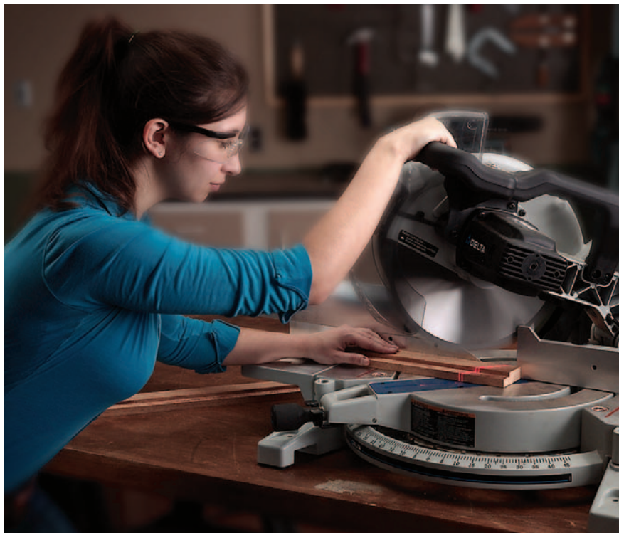
After the tray stiles and rails are cut to width and rabbeted, they can be mitered to length. Use a fine-tooth crosscut blade to help minimize tearout on splintery mahogany.
