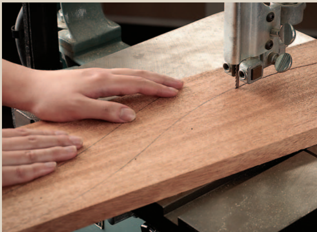
Take the leg blank to your band saw and cut within 1/16" of the line you marked onto the blank. Don't cut into the line; you need to leave some material for the router bit to remove. This will ensure uniform legs.
