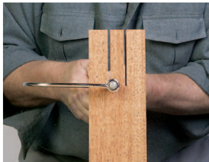
Ian removed the waste in the leg's open mortise with a coping saw.
