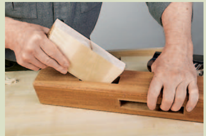
The next step is to check the fit of the wedge blank in your mortise.
