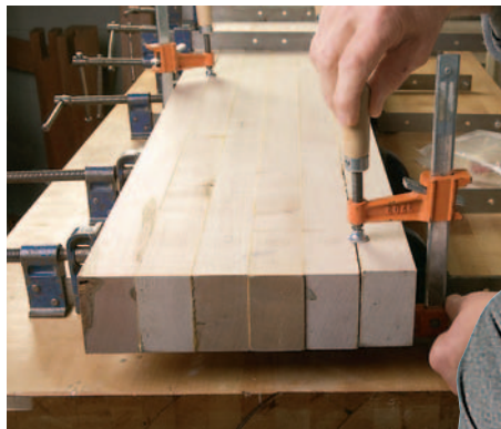
To begin making this elegant and eminently practical bench, start with its top. Glue 16 laminations together to create a solid and stable surface.
