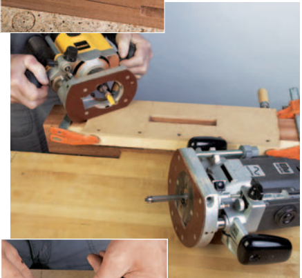
Clean up the mortise with jig-guided router bits. The insert (left) lets you cut two sizes with the same jig.
