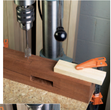
Use a 7/8" spade bit on-center to leave 1/16" of waste on each mortise wall.
