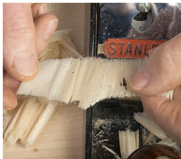
Cross-grain planing produces these typical "fold-up" shavings, which are thick in the middle and thin at the edges due to the curve in the plane blade that prevents plane marks. Clearly evident is the glue line that connects the two laminations.
