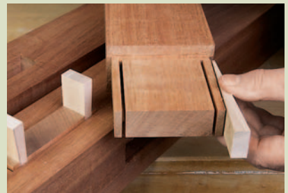
When testing the wedge for fit, don't drive it home! You should be able to see that the length and slope will correctly fit the kerf and opening.
