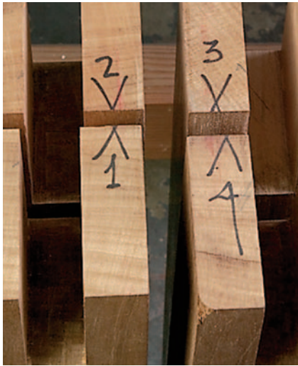
Locate the numbers so they are undisturbed when the joints are cut. The numbers read clockwise and are marked on the side where the long rails meet the legs. The arrows point to where the short rails meet the legs.
