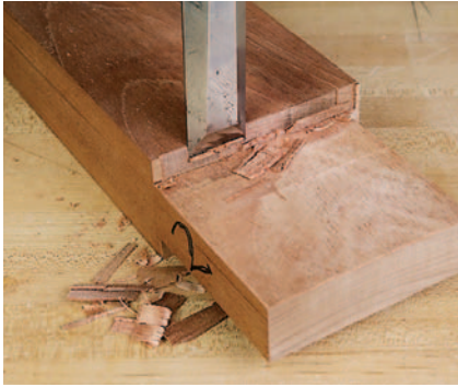
Slower is surer: knife the shoulder lines and clean up with a wide and sharp chisel.
