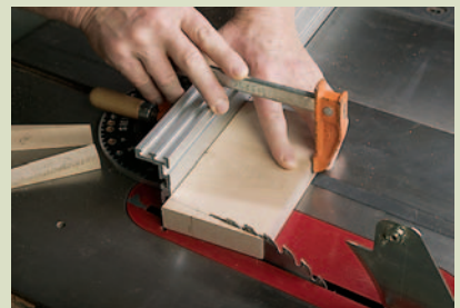
Clamp the blank to the miter gauge fence set at the correct angle and saw a wedge with a 3/32" blunt end. You need a second miter fence set to 90° to saw a second wedge.
