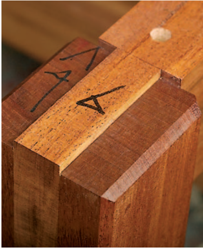
The rail numbers match the leg numbers. Top rails are marked on the top edge and bottom rails on the bottom edge.
