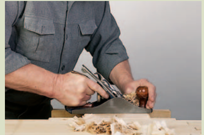
Place a wide maple board, 4" long, on support blocks in the vise and plane across the grain to dimension.
