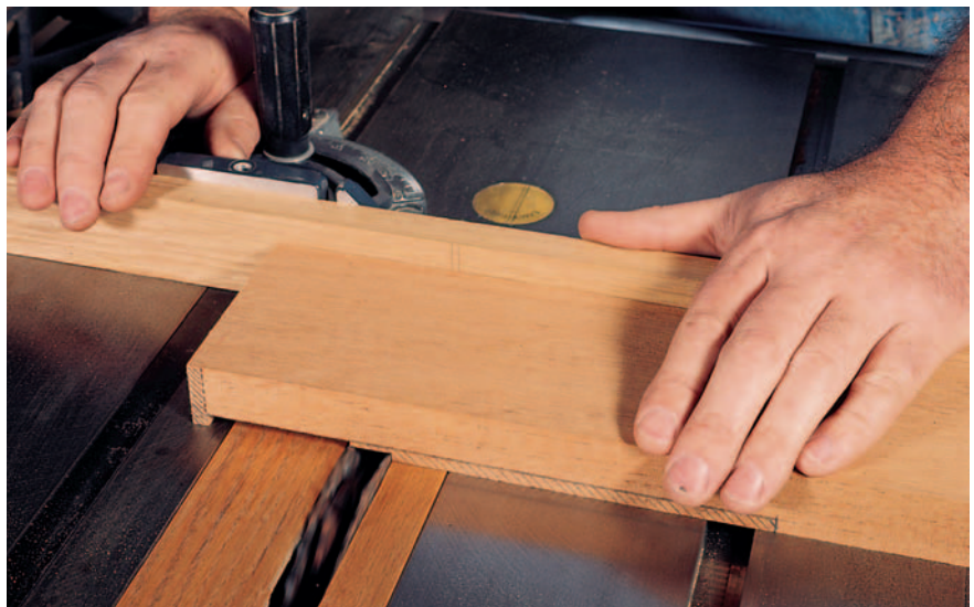
Expose 3/16" of the dado head cutter, then relieve the front face of the plate. Since the length of this dado exceeds half the length of the workpiece, leave a stub at the end to keep the wood from tipping into the blade as the dado gets wider.
