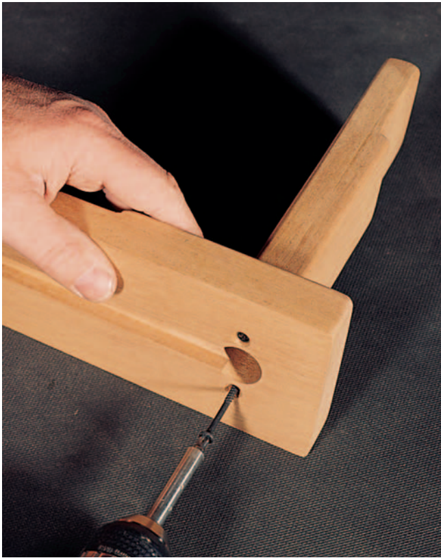
Screws attaching the arm and plate should barely slip through the holes in the plate. The holes in the arm are about half their diameter.
