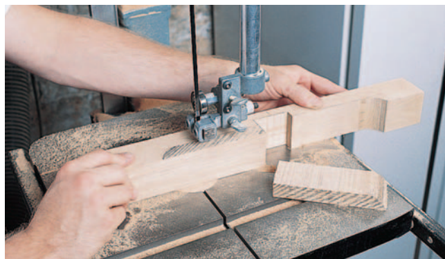
Once the dados are cut, move to the band saw to remove the waste at the bottom of each foot. Then template-rout the final shape.
