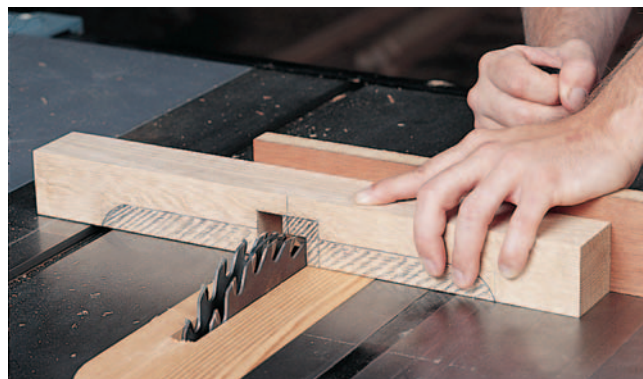
The lap joint dados on the feet are cut first. Clearly mark your stock, and remember to reset the blade height for the second foot.
