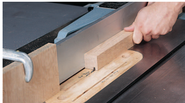
With a stop block in place to create a 7" spline groove, cut the right side of each leg, then reset the fence to cut the opposite sides.
