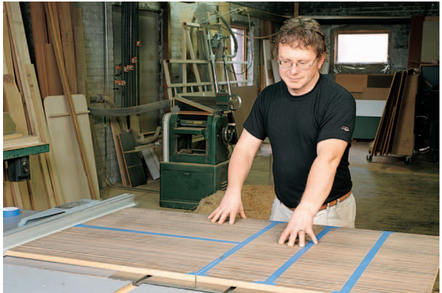
No room for error: If veneering the face frames is the most difficult part of this project, cutting the veneered front panel into doors and drawer fronts surely is the most nerve-wracking.
