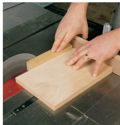
The author installed a disk sander in his table saw, in combination with a miter gauge jig, to taper the Avonite "toes," which must match the leg tapers. Here the author tests the setup with scrap lumber.
