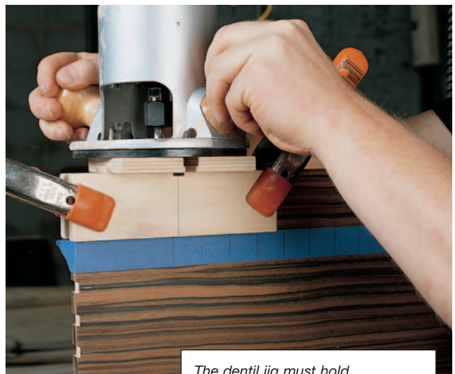
The author made this precise jig to form the dentil-inlay openings. Indexed off of centerlines, the jig surrounds the sides and the edge of the pediment to prevent blowout. Once it's lined up with marks on the blue tape, the jig is clamped in place for each rout.
