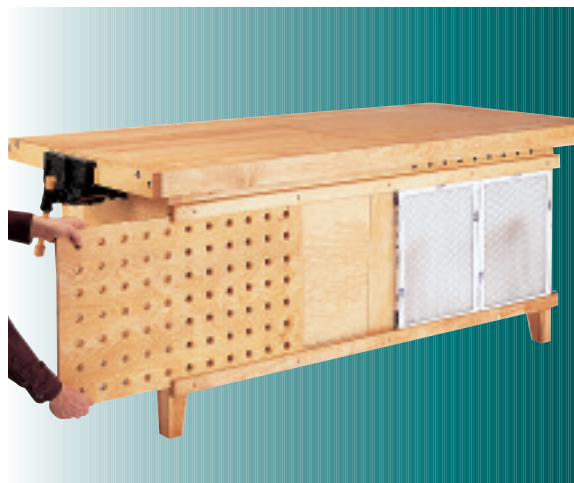
The worktop of this bench has two inserts that fit into a rabbeted opening over the downdraft unit. When not in use, either insert can easily be stored on the back face of the bench.
