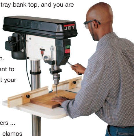
With two stops established on the fence, drill the holes to mount the drawer pulls.
