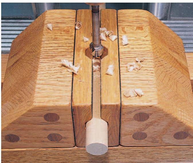
With magnets to hold this drill press vise in place and a variety of clamping options available, drilling dowels and circular-shaped objects is a breeze. We used oak to ensure strength and durability.
