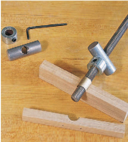
The operating hardware for this drill press vise is a double threaded spindle (allowing both jaws to be driven by a single handle) teamed up with spindle nuts and collars.
