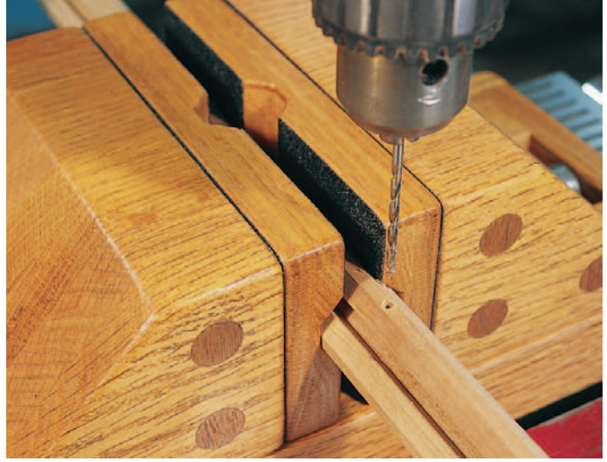
Use a single liner or both at once to effectively grip and secure a wide variety of moldings or other shaped pieces. Even difficult end grain drilling is made easy with this vise fixture.
