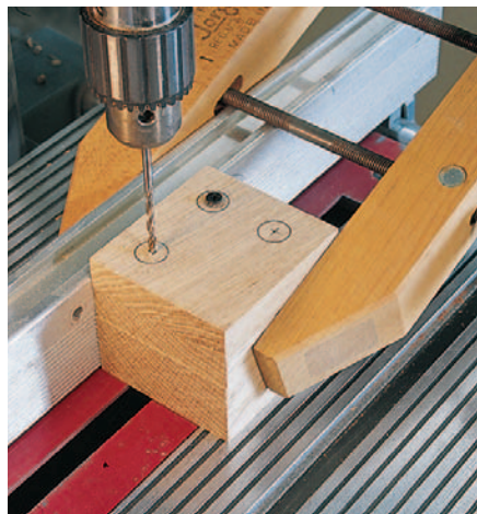
Figure 1: Make the laminated oak sliding jaws first. Stack the jaw parts and machine them while they are still rectangular in shape.
