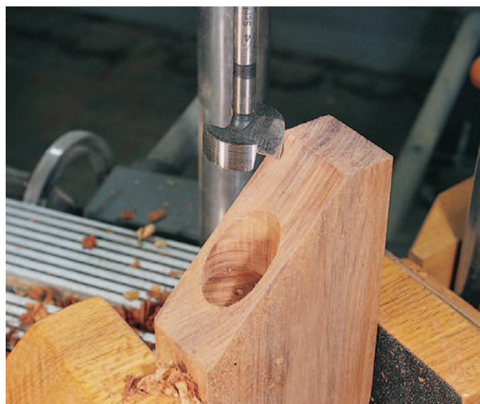
Drilling odd-shaped stock is easy with this drill press fixture. The double threaded spindle allows for single-handed adjustability, and the overall stability adds a level of safety to drilling operations.
