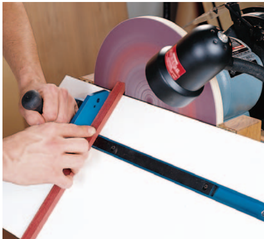
By adding a miter gauge slot, this shop-built disc sander can help create compound angles.
