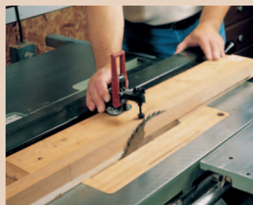
Use this safe, simple jig to cut accurate tapers on your table saw.
