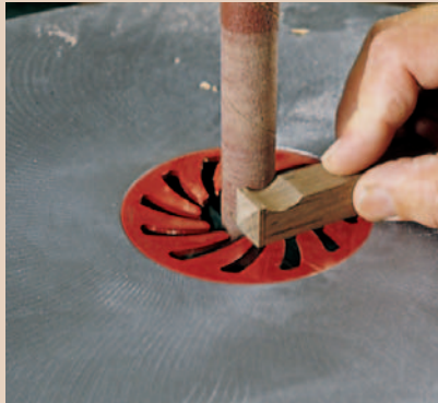
Spindle-sand the the inner contours to shape, then bandsaw the knob free.
