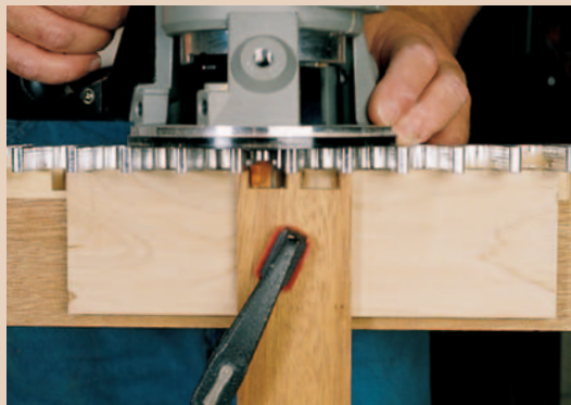
Use the Keller Jig to machine the drawer front and back first, forming the half pins at each end and then centering a pin in the middle.
