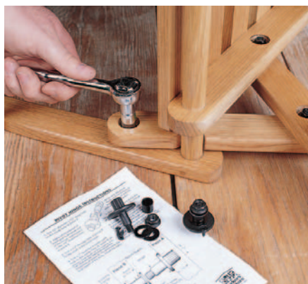
Figure 3: Installing the weather-resistant pivot hinges is a simple matter of lining up the two sides of each hinge and bolting them together.
