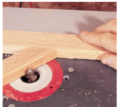
Figure 2: Various elements of the back leg assembly are rounded over with a 1/4"-radius router bit. These cuts are stopped.
