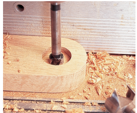
Figure 1: The holes in the seat supports for the pivot hinges are drilled in two stages, changing from a 1" bit to a 1/2" bit.
