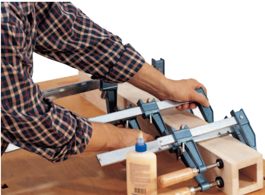
The legs are a glued-up hollow construction. Because the plan was to paint the base, we used yellow poplar, a stable wood that accepts paint well.
