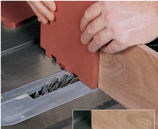
Figure 2: Finger joints are a strong and attractive drawer joining option. A dado head and a miter gauge with a keyed fence register each finger joint accurately. Always test your setup on scrap lumber to avoid problems.
