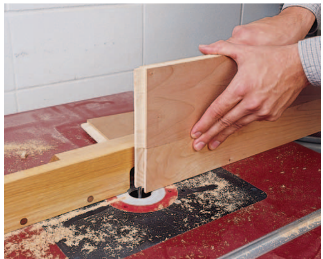
Figure 1: Plow grooves into the appropriate edges of the rails and glued-up rails. Take a few passes to achieve the proper depth.
