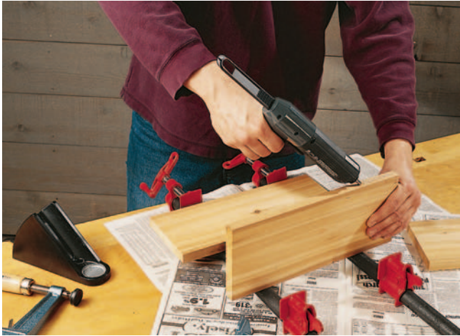
We used Franklin's hot-melt polyurethane for assembly, but any water-resistant glue should work fine. Titebond II or III would work also.
