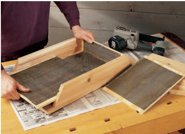
The mesh-covered partitions create an ideal bat roosting habitat. Glue and nail the partitions in place.
