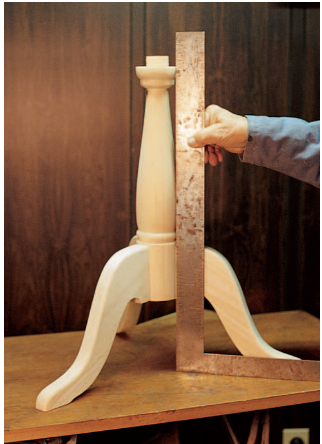
During the final glue-up of the legs to the pedestal, check for plumb with a carpenter's square to be sure there will be no tilt to the top.
