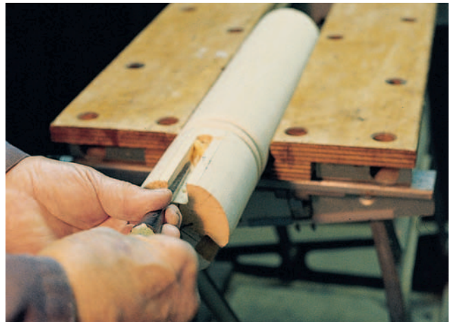
Once the straight bit has done its work, use a sharp chisel to complete the dovetail walls and to flatten the areas that will later be covered by the ends of the legs.
