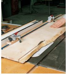
The hold-down option on this jig allows you to slice straight edges on rough stock without fear of binding or kickback.
