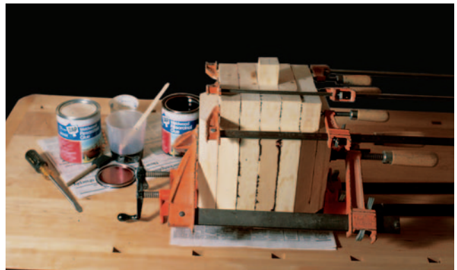
Figure 1: Clamp the birdhouse together by turning the assembly upside-down and setting it onto two bar clamps. Add more clamps as needed.
