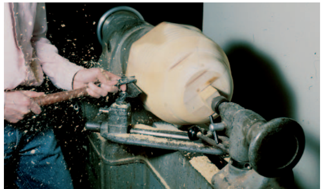
Figure 2: Use a large roughing gouge and run the lathe at a very low speed to turn the blank into the apple shape.
