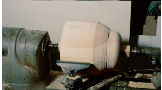
Figure 3: The wall is thinnest at the shoulder near the bottom of the apple, so it's important to keep this area marked to prevent overcutting.
