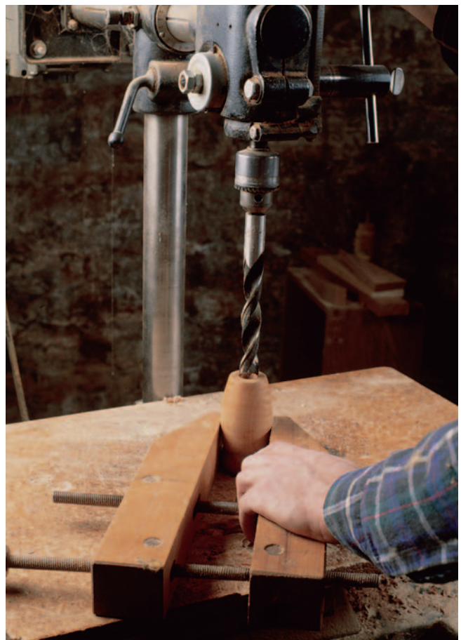
Figure 1: When you're ready to drill the cores, a wooden handscrew clamp will help keep the mill from spinning during drilling as well as align the workpiece for an accurate through hole.
