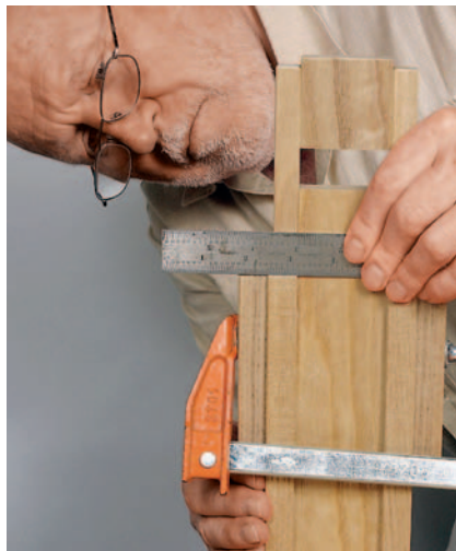
Figure 15: Glue and clamp the short shoulder rail flush to the shoulder rail.
