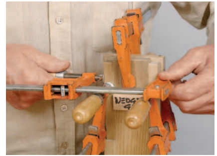
Figure 10: Position, clamp and glue the mortise block between the rail extension strips with the aid of an alignment block (at rear) and a wedge spacer strip.
