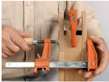
Figure 9: Position, glue and clamp rail extension strips with the aid of an alignment block.
