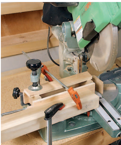
Figure 18: Clamp the jig tight to the bed and fence of the chop saw. Holding it by hand is neither safe nor accurate.
