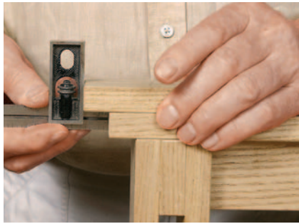
Figure 8: Position the overhang of the foot piece using a sliding head square, then screw into place.
