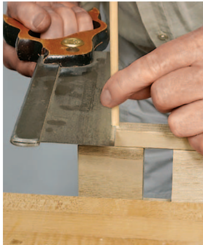
Figure 13: Saw off the excess length of dowel before cleaning flush with a chisel.
