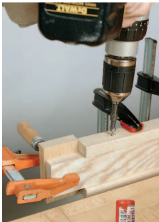
Figure 11: Position the first shoulder rail on the stretcher rail with a screw at each end, then glue and clamp in place.
