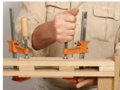
Figure 6: Glue and clamp the outer leg to the leg blocks.
