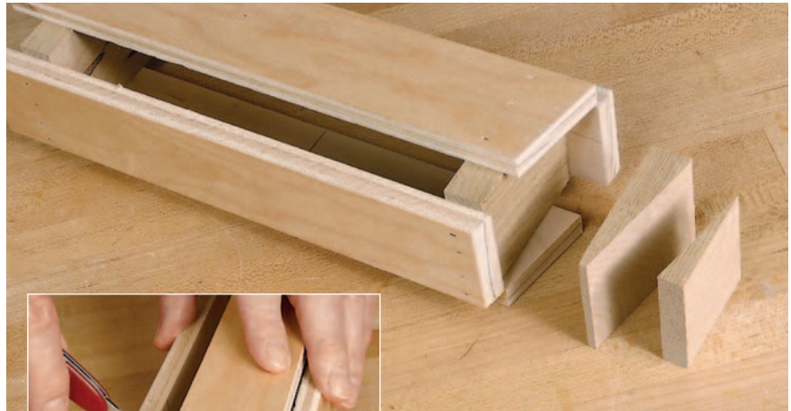
Figure 17: Make the wedge jig using two wedge blanks and strips of 1/2" plywood. The narrow strips allow access to the corner of the wedge to pry it out after cutting (see inset).
