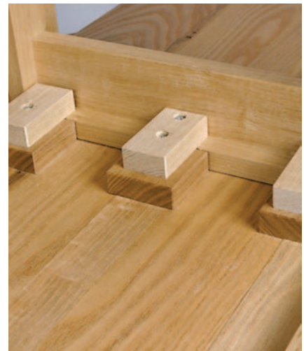
Figure 19: The top is secured and fixed on center by blocks that trap one flange of the cap rail while allowing for shrinkage and expansion.
