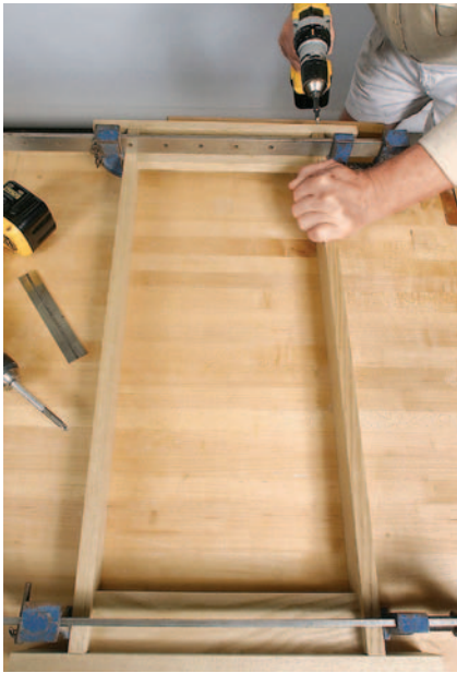
Figure 3: Clamp the shoulders tight to the cap and shoulder rail assembly with the inside legs in place.
