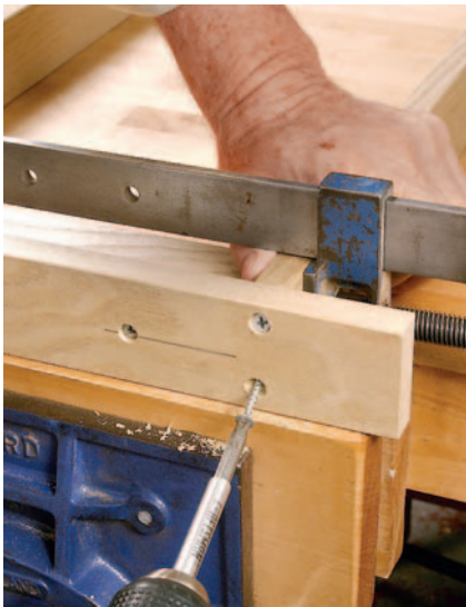
Figure 4: Screw through the cap rail into the end grain of the inside leg. Screws are angled towards one another for extra strength.
