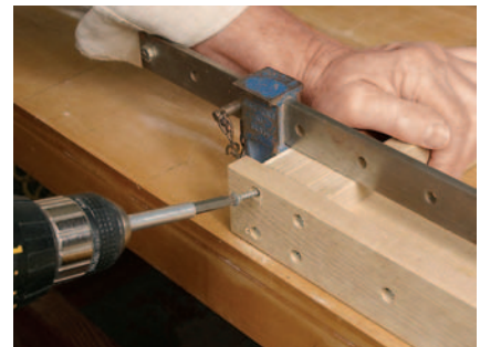
Figure 7: Glue and clamp outer legs to the leg blocks, then screw them through the cap rail.
