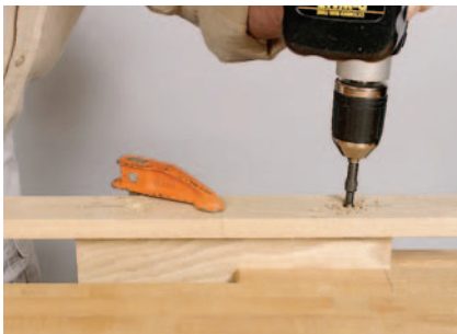
Figure 2: Clamp, drill, and screw the parts together dry to assist with positioning them once the glue is applied.
