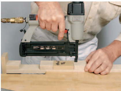
Figure 5: Glue leg blocks, avoiding squeeze-out, then screw or staple into place. Position center leg blocks using the 3/4" spacer.
