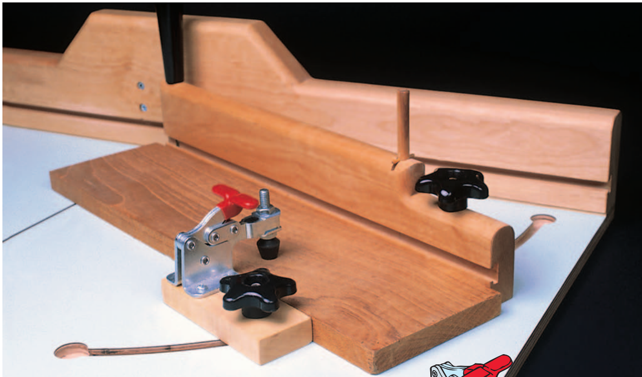
Figure 4: While mitering, boards sometimes creep along the fence and spoil the cut. Using the hold-down jig solves the problem entirely.
