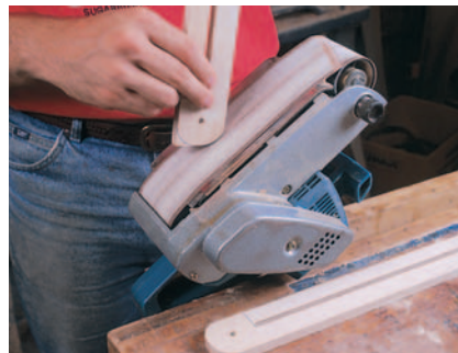
Step 5: Secure your belt sander in a vise and shape the ends of the adjusters. Use a palm sander to smooth the jig's surfaces and ease all the corners. Apply a coat of sanding sealer.
