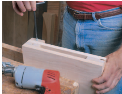
Step 2: Drill pilot holes for the threaded inserts in the ends of the strips, screw blocks and in the bottom plate. Wax the inserts and install them with a hex driver.
