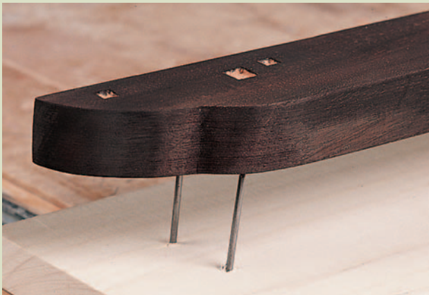
Drive several nails up through a piece of scrap to support your workpiece while it dries.
