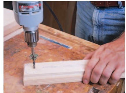
Step 3: Cut plywood for the adjusters and lay out the pivot hole and slot on each one (see the Elevation Drawing on page 58). Drill the 1/4" pivot holes.
