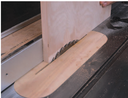
Step 1: Cut stock to size and rabbet the lower plate and one strip to accommodate the hinges (see Hinge Detail, page 59). Secure the hardwood to the plates with screws and install the hinges.
