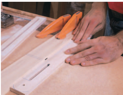
Step 4: Rout the slots in shallow passes with a 1/4" straight bit after marking the bit's cutting area on the fence. Use the marks as guides for starting and stopping the cuts.
