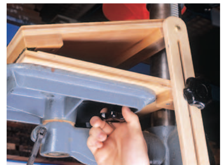
Step 6: Bolt the adjusters to the upper plate assembly and clamp them to the screw blocks with knobs. Use the remaining two knobs to secure the jig to your drill press table.
