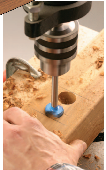
Figure 1: Drill out your mortises with a 1½" Forstner bit, using a fence to keep the holes aligned in the center of the piece.
