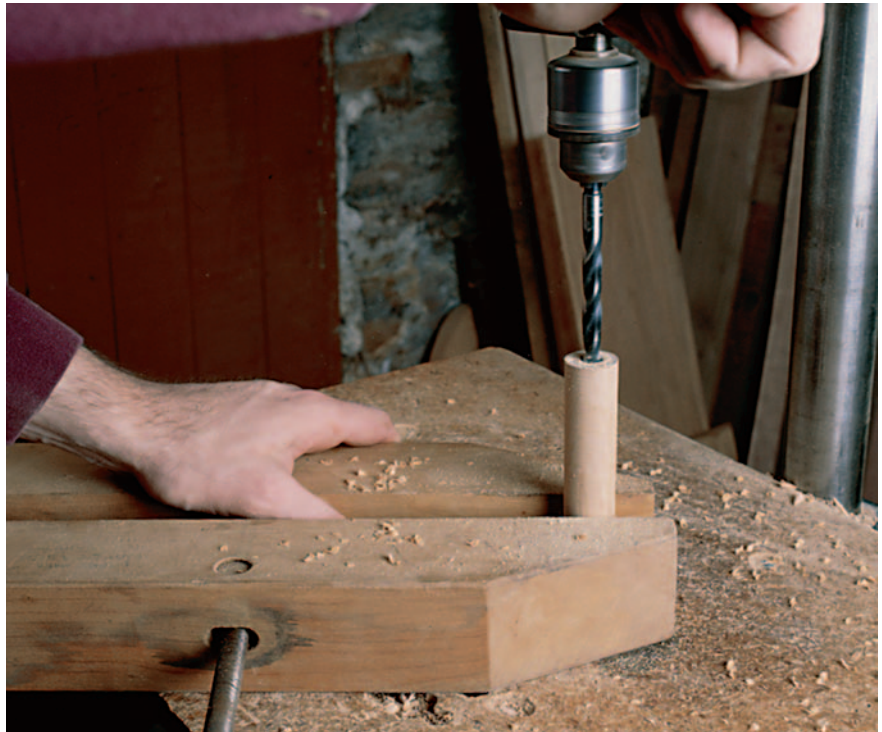
Figure 1: To ensure straight holes in the handle and washers, use a wood handscrew clamp to hold the dowels square to the drill press table.
