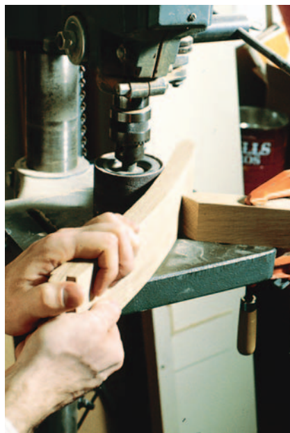
Figure 1: Create uniformly sized and smoothed curves by pushing the stock between a V-block and a sanding drum mounted in a drill press.
