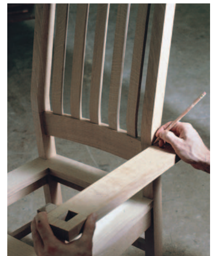
Figure 3: Align the arm mortise with the front leg tenon and rest the arm on the shoulder. Lay out the rear joint where the arm intersects the back leg.
