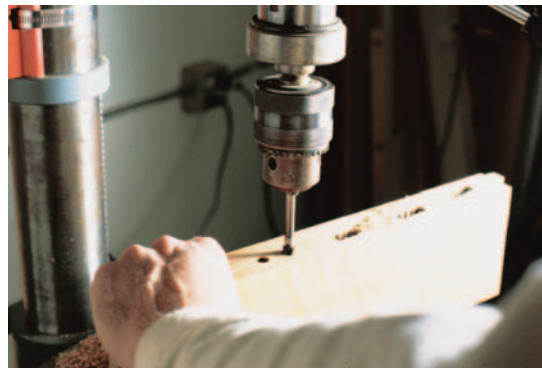
Figure 2: Use the drawing below to lay out all the angled tenons in the project. Hollow out the rail mortises with a 3/8" drill bit, then clean up the mortises with sharp chisels.
