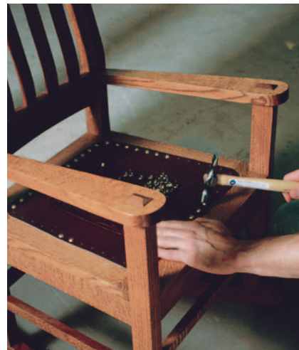
Figure 6: Trim the leather to lap onto the side rails by 1" and 2" on the front and back rails. To prevent splitting, drill pilot holes for the nails 1" apart.
