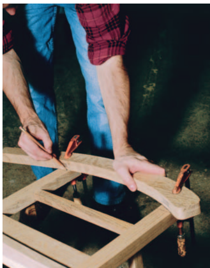
Figure 4: Position the rocker on the legs, then trace the curve to lay out the tenon shoulders accurately.
