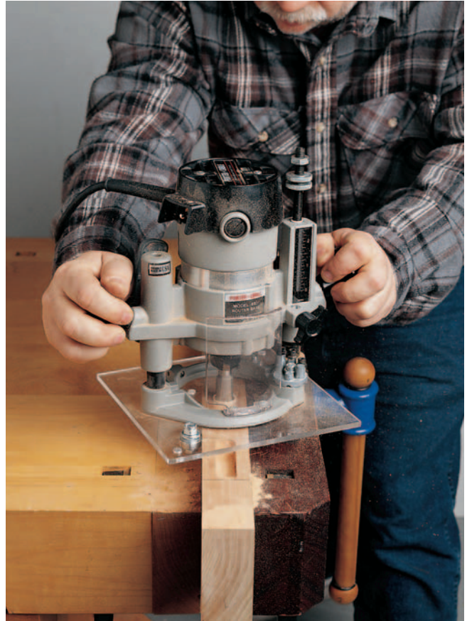
Drill extra bearing guide holes closer together for mortising narrower stock. This allows you to get closer to the ends of a board.
