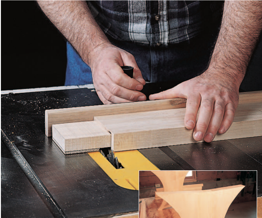
Figure 2: Dry-fit the stretcher in the leg mortises to ensure a perfect fit. To define the tenons, use a sharp, fine-toothed blade, and then reveal the cheeks with a dado set.
