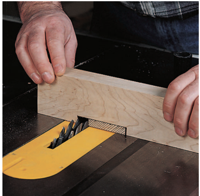
Figure 1: The split mortise in each leg is created by ripping stock down the center, dadoing half the mortise out of each piece, and regluing.
