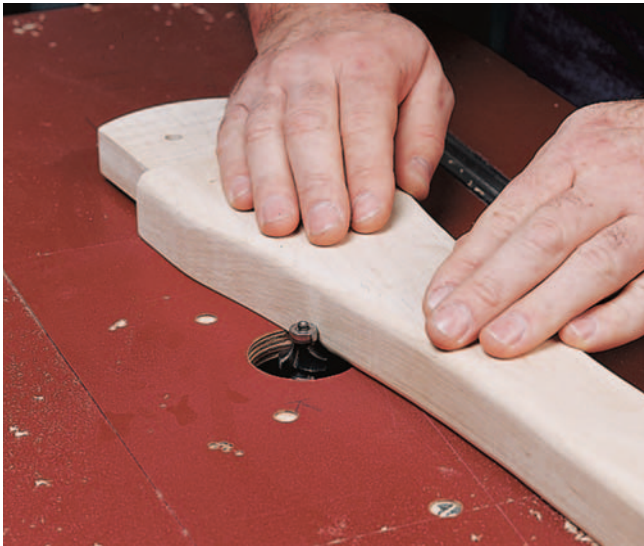
Figure 3: Most of the edges of the split mortise bench are rounded over with different bits prior to final assembly.
