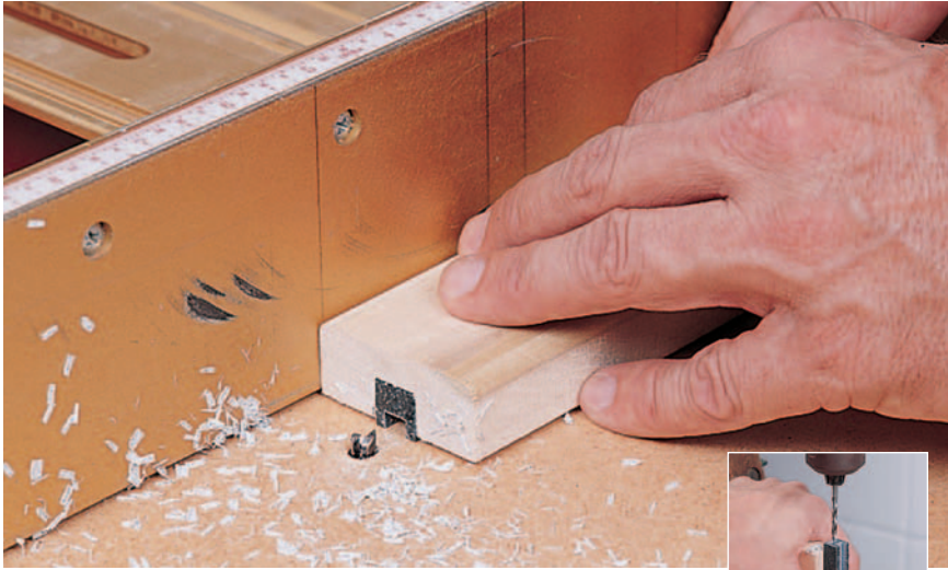
Figure 1: A scrap sled keeps the routing operation safe and creates perfectly centered cuts on each frame piece. Once the sides are dadoed, a fence and stop block on the drill press (right) ensure accurate holes for the studs.
