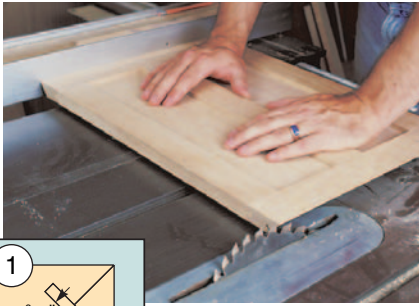
Figure 2: When cutting the spline grooves, once again use 1/4" strips to balance the side panels.
