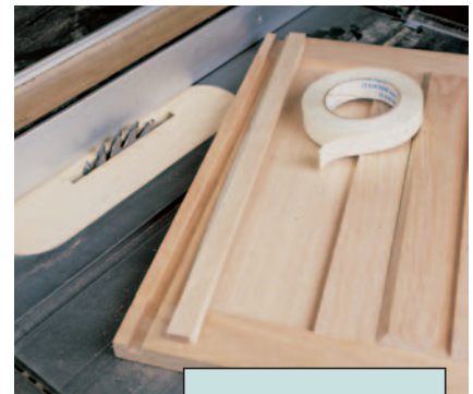
Figure 1: For balance, tape a 1/4"-thick strip to the side panels when making the bottom groove dado cuts.
