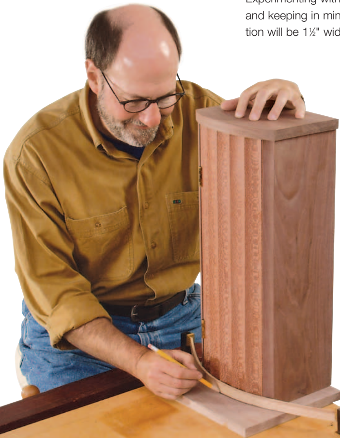
The author scalloped the front edge of the sides on his router table (above). A 1/8" strip of hardwood, flexed on his workbench or between a pair of nails, will provide a perfect offset for the top and bottom and make it easy to transfer the curved shape.
