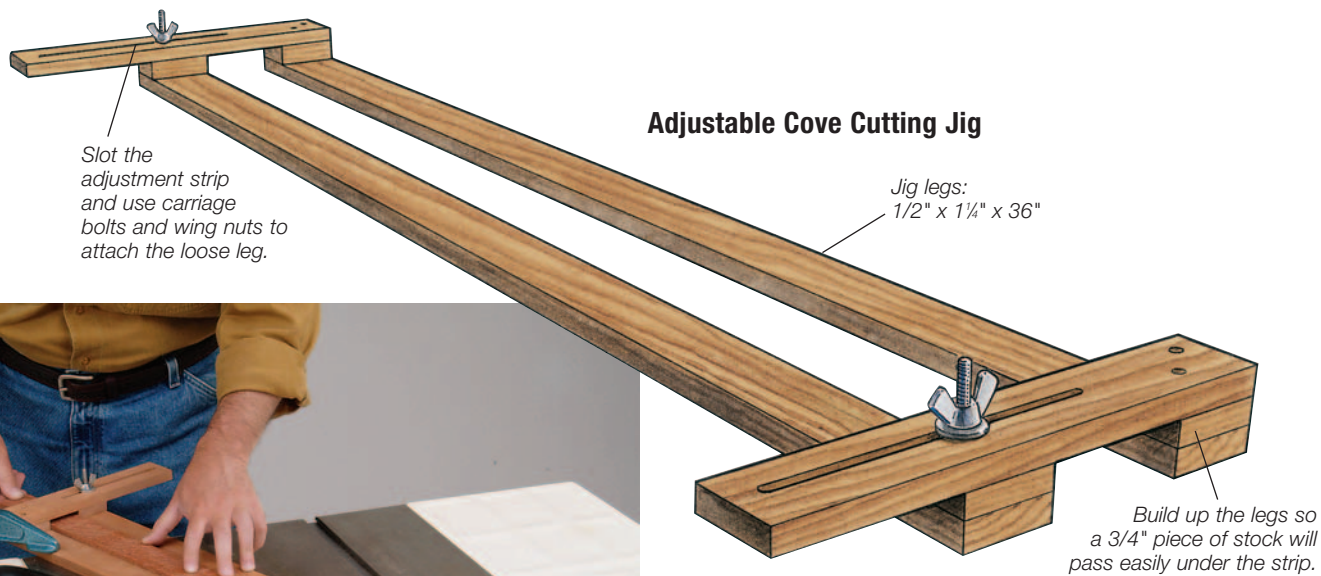
After many test cuts on pine, the author used his shop-made jig to form the coves in the lacewood staves. The adjustable jig accommodated both widths of door staves.
