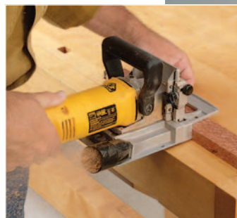
After plowing the coves on each door stave, the author formed a 5° angle on both long edges (with the exception of the outside staves). To align the staves during glue-up, biscuit joints were put to good use.
