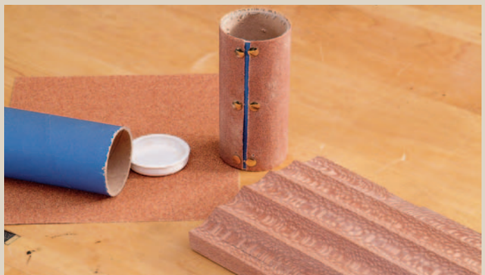
The radius of a mailing tube was key to the author's success in creating his dramatic door with knife-edge arrises.
