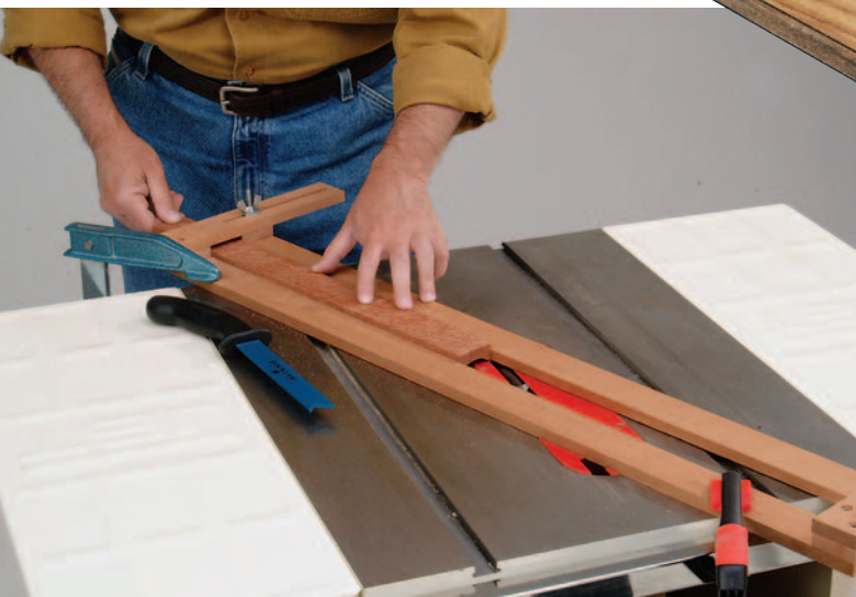
After many test cuts on pine, the author used his shop-made jig to form the coves in the lacewood staves. The adjustable jig accommodated both widths of door staves.
