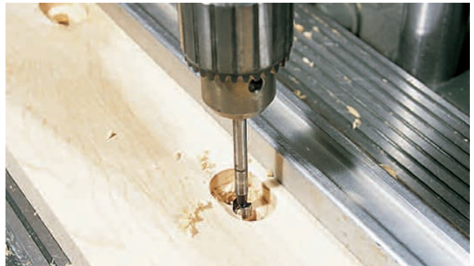
Figure 3: Use your drill press to bore two step slotted holes in the endcaps: these will allow the benchtop to adjust to various levels of moisture in the workshop.
