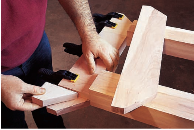
Figure 4: Dry-fit the legset parts together, then use this as a template to determine the shape of the foot and top inserts.
