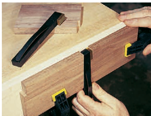
Figure 2: Dry-fit the bench dogs and spacers, leaving gaps that are the size recommended by the dogs' manufacturer. When everything fits, trim the final spacer to length.
