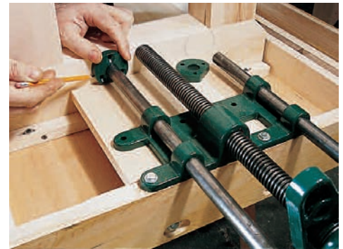
Figure 5: The vise attaches to both the endcap and vise support. With two screws holding the unit in place, establish the locations for the guide rod and center screw holes in the legs.
