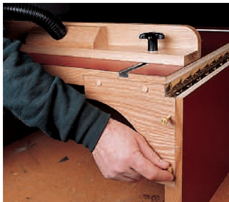
Figure 2: Gussets that are mortised into the back of the tabletop allow the top to be converted into a portable benchtop unit.
