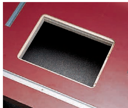
Figure 1: The router table insert rests on a rabbet that holds it flush with the tabletop. Follow the instructions that come with your plate for cutting this opening and rabbet.
