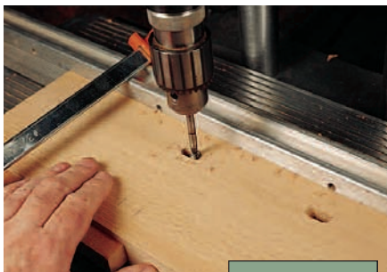
Figure 3: The glued-up tabletop will expand and contract to a significant degree. Oblong slotted screw holes allow that movement to take place while firmly securing the top to the leg sets.
