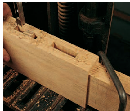
Figure 2: A dedicated mortising machine will make short work of the many mortises featured in this project's Stickley-inspired joinery.
