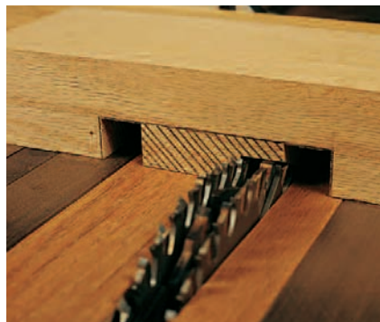
Figure 1: The leg mortises are formed before the legs are glued up. Simply slice wide dados to form one half of each mortise.
