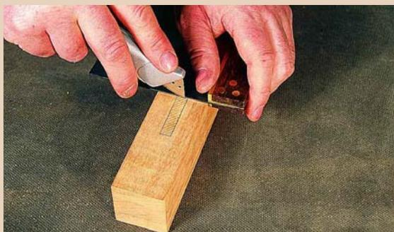
After laying out the matching mortises in the legs, score them with a sharp utility knife to avoid tearout as you drill.
