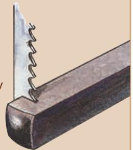
Cut the splines (pieces 13) to the shape found on the *Pinup Shop Drawings*. Again, use a sander to help create the gently rounded profiles on the splines. Move to the buffing wheel and repeat the buffing technique you used on the plugs. Polish the Ebon-X smooth as silk, bringing it to a high, rich luster.
