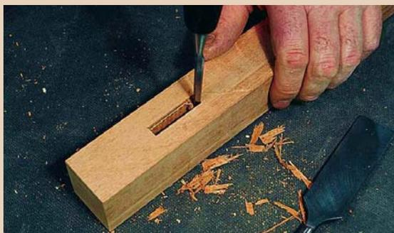
Clean up with a sharp chisel, cutting across the grain on the top and bottom first, then with the grain along the sides.
