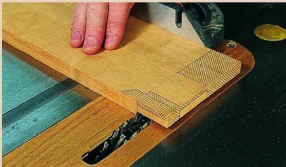
Before cutting the shaped profile on the top center aprons, reveal the tenons on their ends using a dado head in your table saw.
