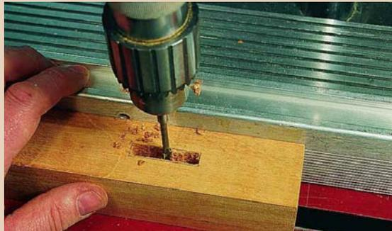
A Forstner bit chucked in your drill press will remove most of the mortise waste, and the bit's design leaves a nice, flat-bottomed cavity.
