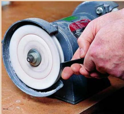
Polish the Ebon-X plugs and splines to their final luster with a polishing wheel mounted in a bench top grinder.
