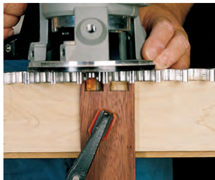
Both drawers have through dovetails and plywood drawer bottoms. Test your setup on scrap lumber of the same dimensions.
