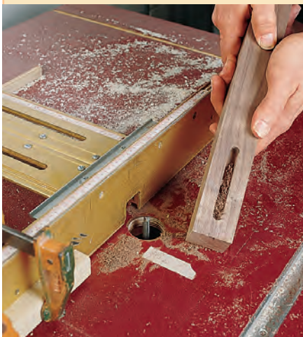
Figure 1: Floating tenons are a unique feature in this design. Use a stop block and masking tape to start and stop your mortises.
