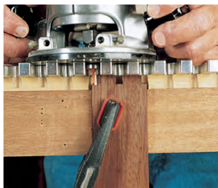
Use a Keller Dovetail jig or similar jig to create the dovetails on the drawers. Be sure to use different size dovetail bits on the large and small drawers.
