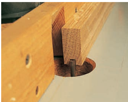
Figure 1: Just about all the tongues and grooves can be cut on the router table with a single fence adjustment.
