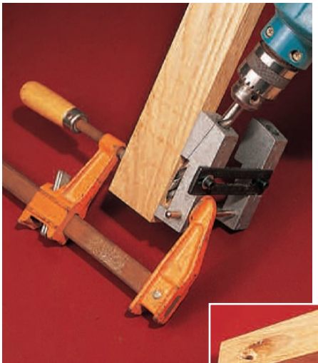
Figure 3: Use a pocket hole jig to create the hidden pilot holes in the three stretcher pieces.
