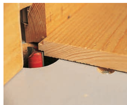
Figure 2: Cut a tongue or groove on all four edges of the redwood panel pieces, and follow up with a chamfering bit.
