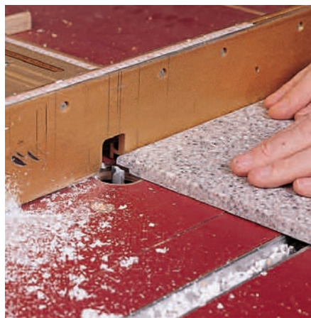
Figure 4: After rounding over the top edge of the Corian with a 1/4" roundover bit, create a rabbet in the bottom edge with a straight bit.
