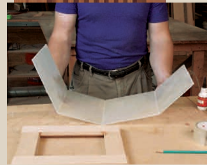
Miter-roll the shade pieces into a cube using 3M packing tape as your hinge. Tape the last open joint closed, then apply a bead of Super Glue along the inside of each joint to bond the parts.
